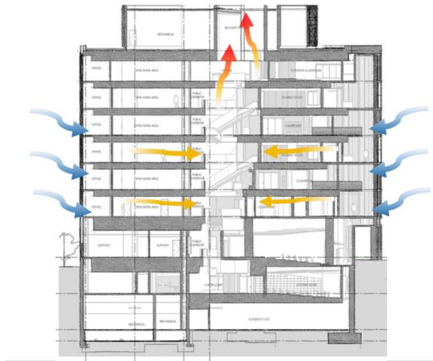
Figure 20: Natural Ventilation Flow through Atrium Space
