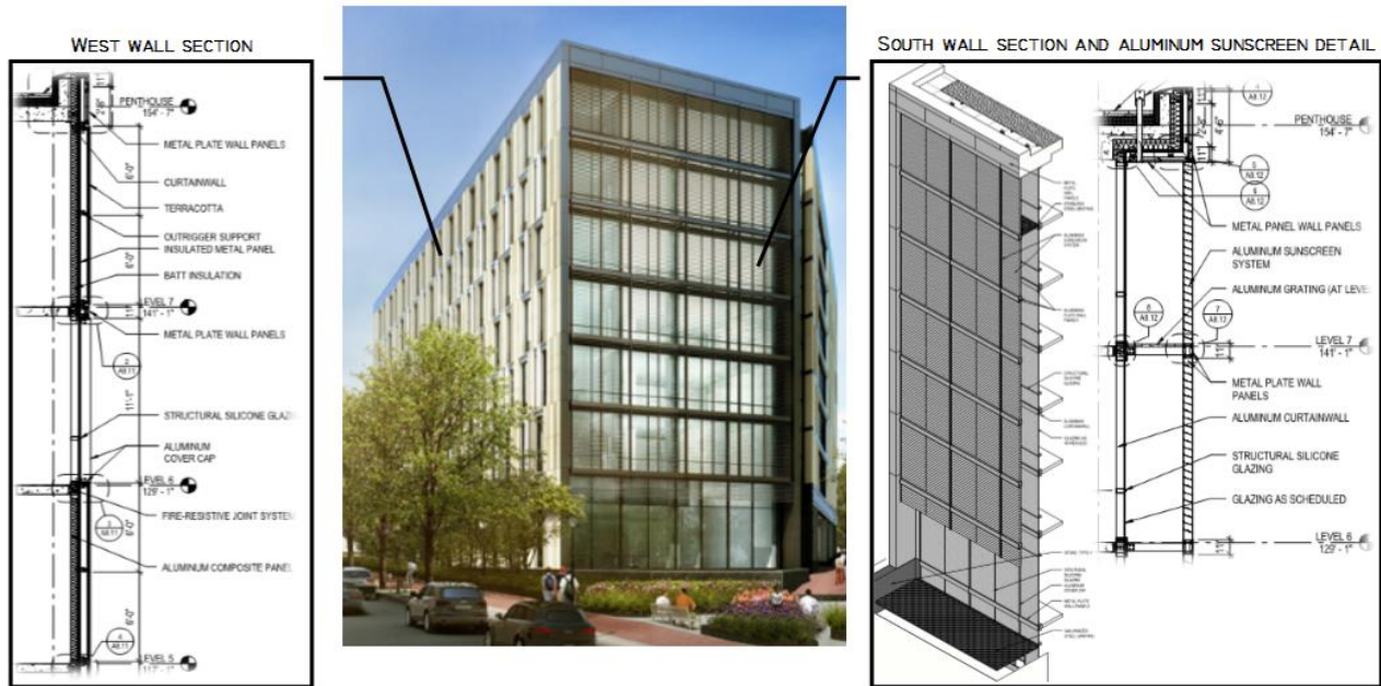
Figure 5.3: West and South façade details
